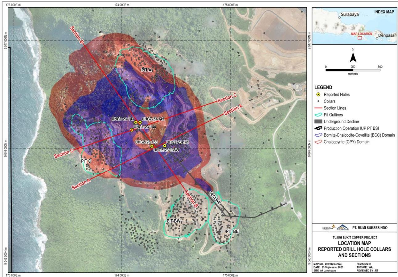
Figure 1: Location map of Tujuh Bukit Copper Project showing reported drill hole collars and sections, Bornite-Chalcocite-Covellite (BCC) and Chalcopyrite (CPY) Domains
