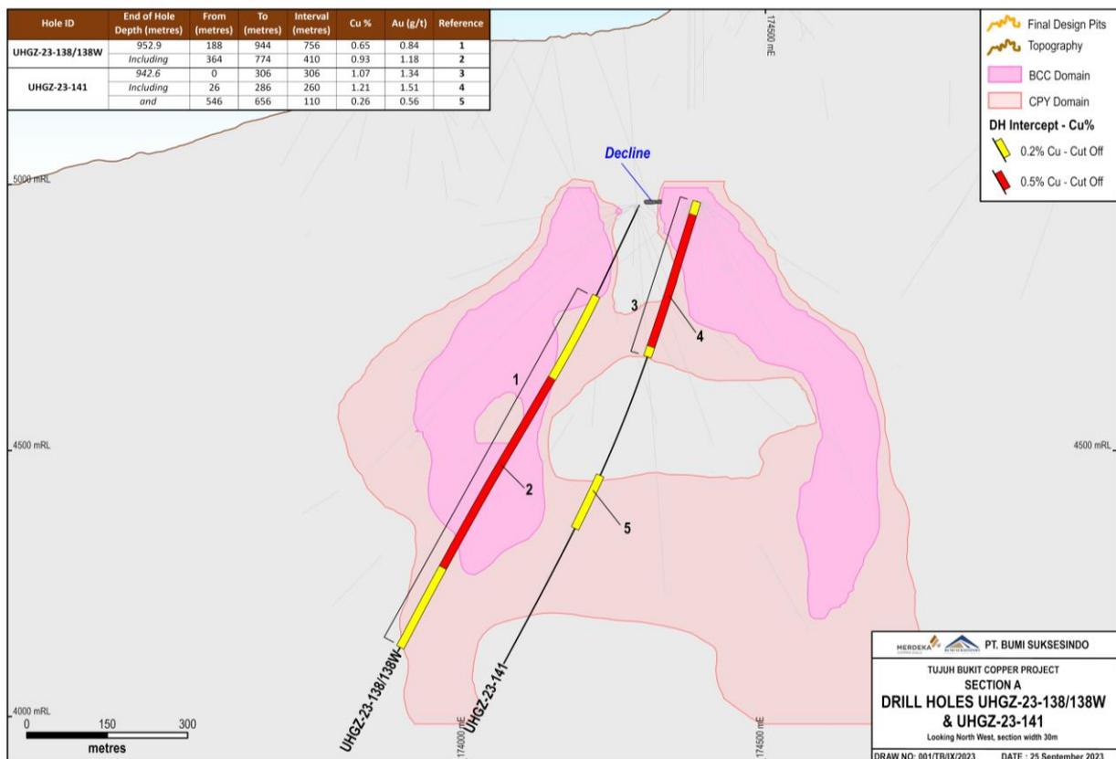
Figure 2: Drill section A, showing drill hole UHGZ-23-138W and UHGZ-23-141 along with mineralised envelopes and drilling intercept information.
