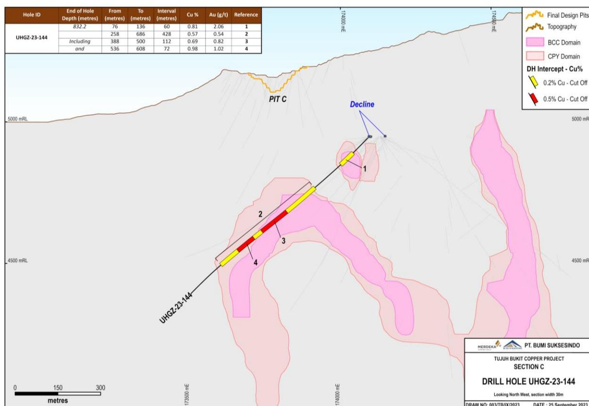
Figure 4: Drill section C, showing drill hole UHGZ-23-144 along with mineralised envelopes and drilling intercept information.
