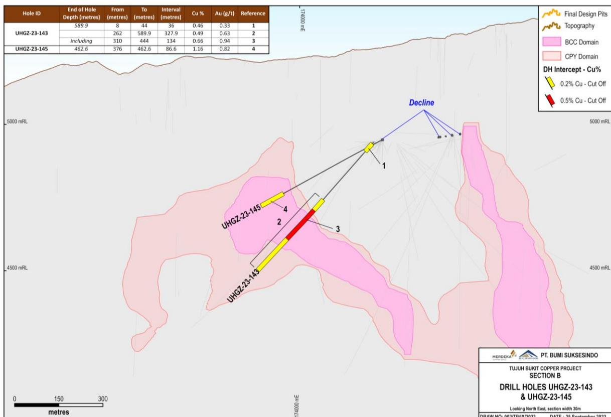
Figure 3: Drill section B, showing drill hole UHGZ-23-143 and UHGZ-23-145 along with mineralised envelopes and drilling intercept information.
